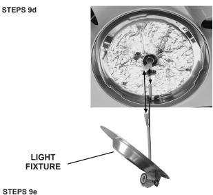
**Step 9e.** Align the light fixture to the three screw holes on the light adapter plate using the light fixture screws, then attach the light fixture to the fan.
